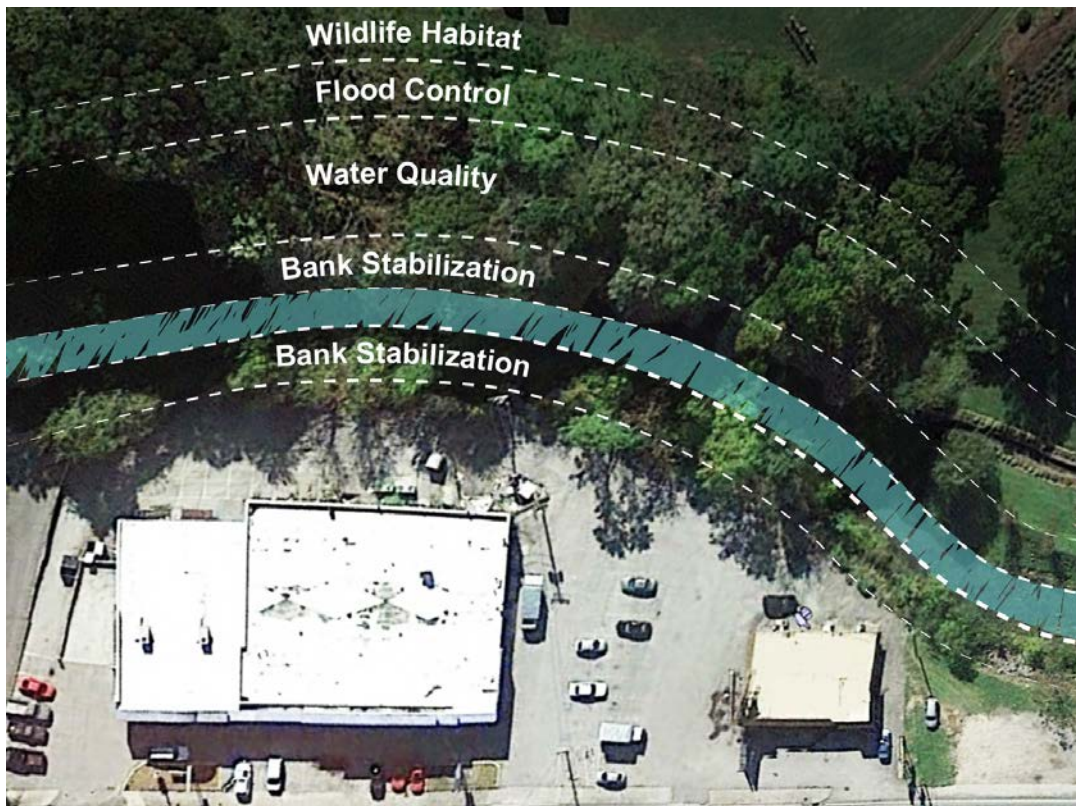
Figure 3. Aerial view of a forested buffer showing that the wider the buffer the greater the ecological benefits (Image ©2014 Google Earth).
